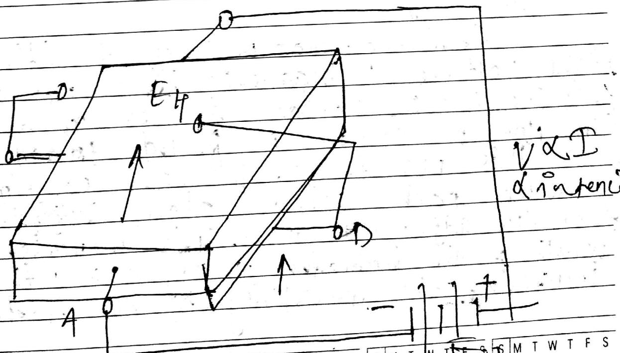
When a current flows through a semiconductor bar placed in a magnetic field a voltage is developed at right angle to the both. If the current & the magnetic field this voltage is proportional to the current & the intensity of the magnetic field this is called as hall effect.
