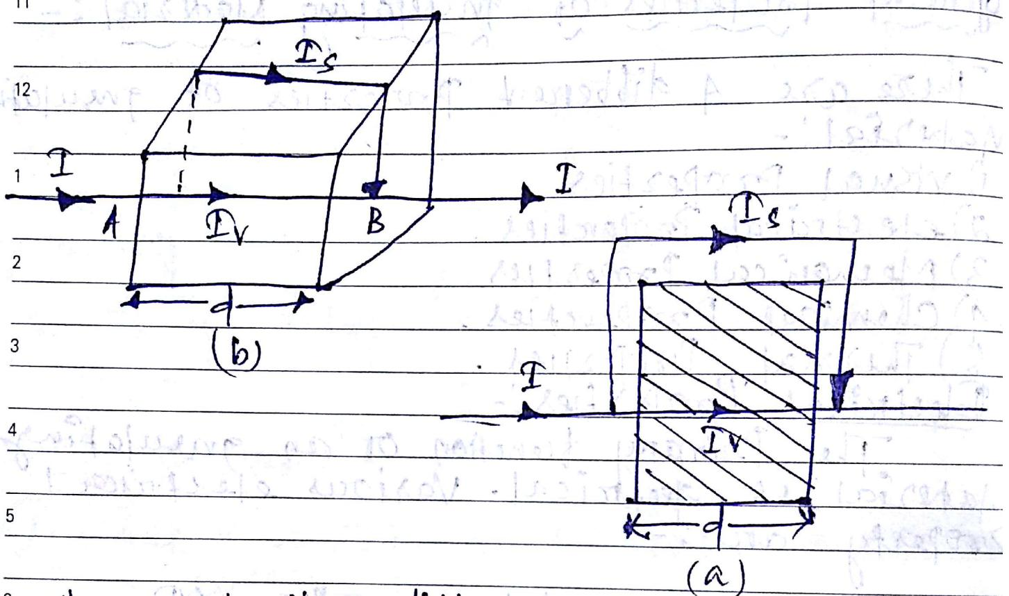
Get a potential difference applied across 'A' & 'B', the current will flow. The current is straight through the material & around the material over the surface. The current that flows through the material is denoted by 'IV' & the current that flows over the surface is denoted by 'IS'.
