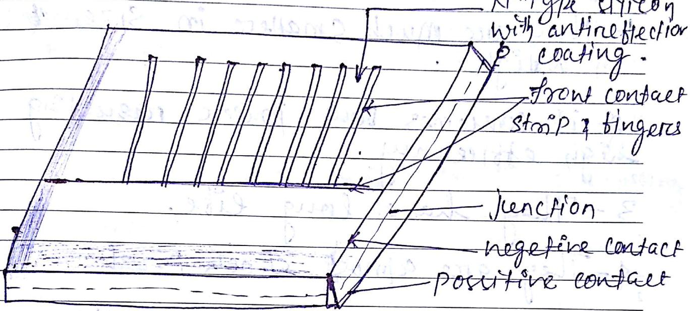
3 Sun is a vast source of energy. One of its important application is the conversion of solar power onto electrical power. This phenomenon is called the Photo voltaic effect. Solar cell is the most important photovoltaic device which directly convert the solar radiation into electrical energy. Solar cell is basically a thin disc of PN junction with a large surface area.
