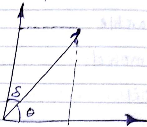
Phase Relation b/w leakage current & applied voltage in Dielectrics.
