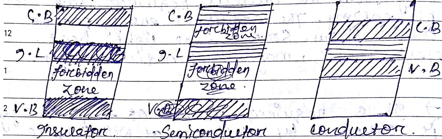
→ The forbidden zone between the valence band & the conduction band is quite large in case of insulator this indicates that electron in valence band required large in case of insulator this indicates that electron in the valence band required large amount of additional energy to move up and becomes free. Long as the valence electrons are unable to move upto the conduction band there can be electron flow.
