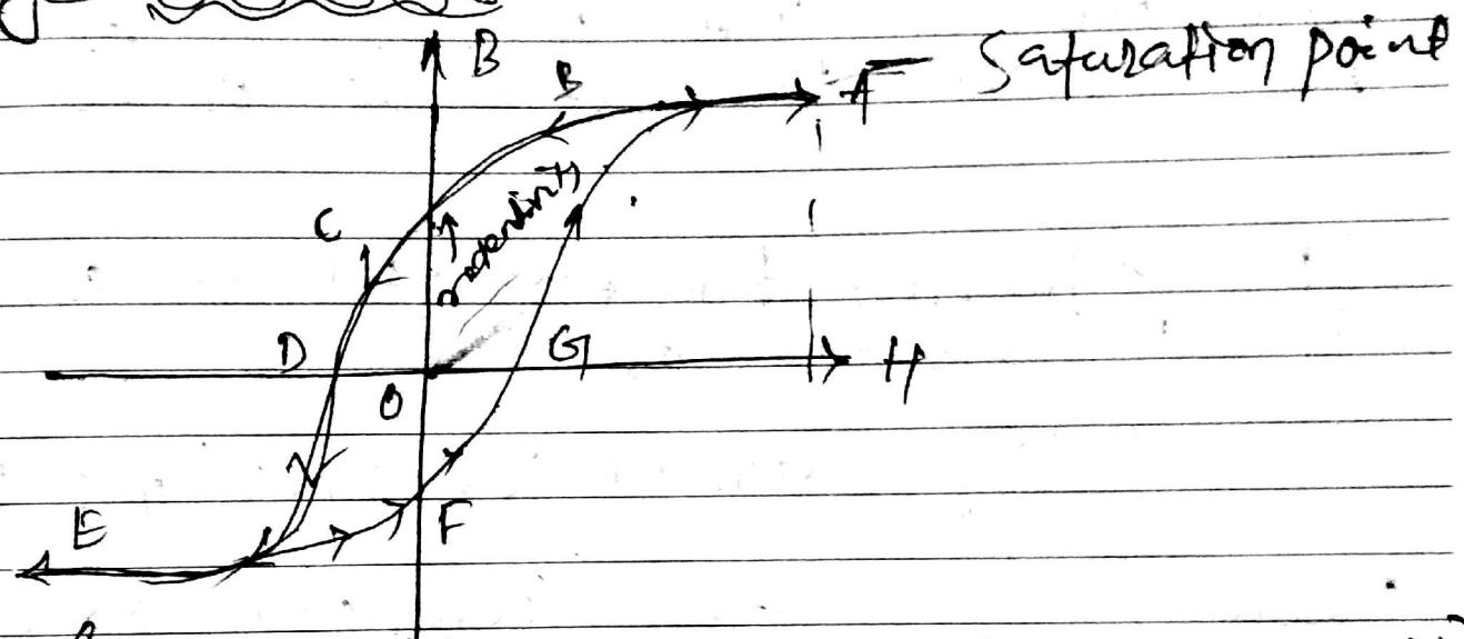
(Hysteresis loop for a ferromagnetic material)
